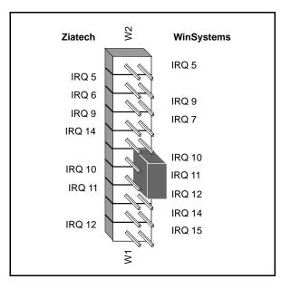
Figure 2-7. Jumper Setting for Disabling Interrupts
